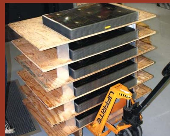
The covers had to be stacked on short lifts to ensure proper drying without distortion.
